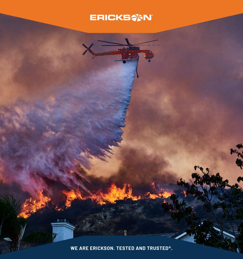
Erickson is proud to be the OEM of the S-64 Air Crane® helicopter, delivering results since 1971. The S-64 is a powerful tool — a precision lift machine that can lift 25,000 lbs.; yet is remarkably agile and maneuverable.
