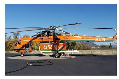
K7, incorporating the latest modifications, including composite made rotor blades and glass cockpit. KFS continues to be a leader in aerial firefighting, utilizing the most robust aircraft, for the toughest job.
