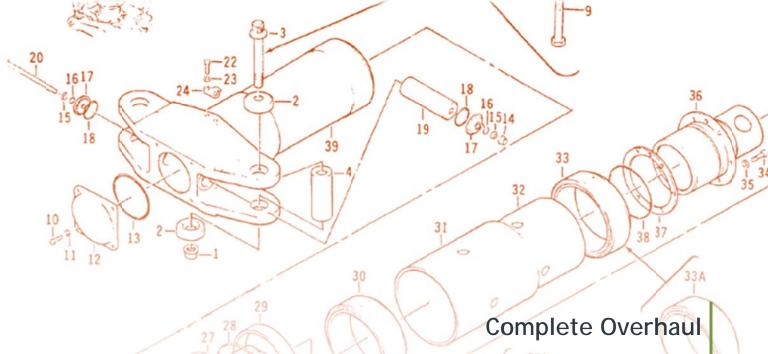
Inspect / NDT / Machine bushings / Inspect strap pin bores / CAD / Bushing replacement per ASB 214-12-73 / Line bore / Mask and apply dry film lube / Prime and paint / Final Inspection and RTS
